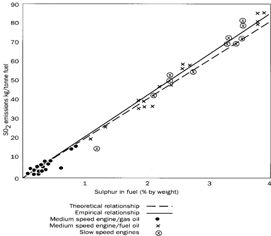
Figure 5 Relationship between fuel sulphur content and SO<sub>2</sub> emissions for marine diesel engines (Lloyds Register 1995)
