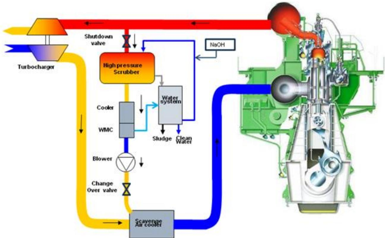
Figure 8 Principles of an EGR system (MAN Diesel)
