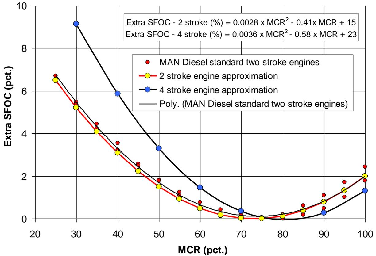
Fig. 3 Variation of SFOC for 2- and 4-stroke engines as function of MCR in per cent (data from MAN Diesel A/S)
