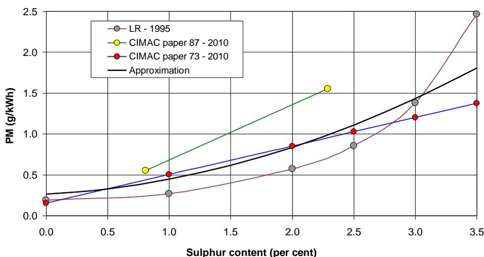
Fig. 9 Relationship between fuel sulphur content and emissions of particulates, PM (Lloyds Register 1995 and CIMAC 2010)
